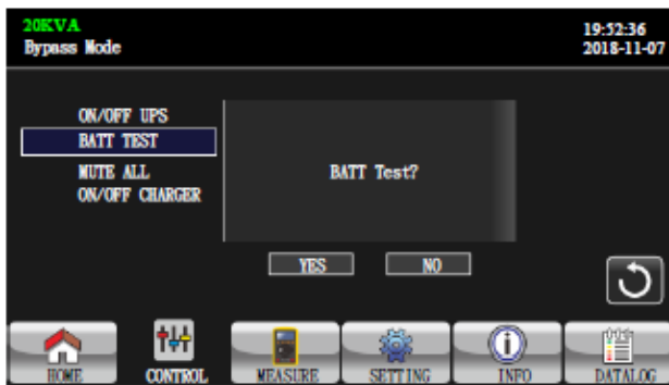
Turn on battery test
